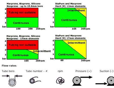
**Note:** Flow rates quoted have been rounded for simplicity, but are accurate to within 5% - well within the normal tubing tolerance variation of flow rate. They should therefore be taken as a guide. Real flow rates in any application must be determined empirically.
