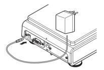
Connect the AC adapter to the connection socket on the back of your balance (see figure) and to the power line.
