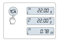
The « key can be used at any time to toggle between weight unit "UNIT 1", "RECALL" value (if selected), weight unit "UNIT 2" (if different from weight unit 2) and the application unit (if any).
