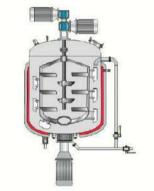
Single way mixing & external circulation Double way mixing & external circulation Single way mixing & internal circulation
