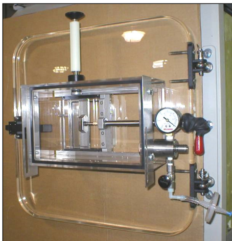
Sample Extractor Assembly Door Without Front Antechamber Cover And Selector Arm.
