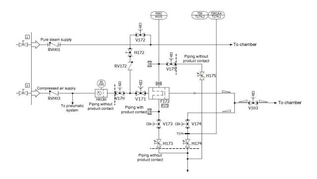
The equipment consists of the necessary piping including fittings as well as the corresponding software to perform an automatic inline filter sterilization of the compressed air filter. See chapter "Automatic inline filter sterilization" for the recipe sequence.
