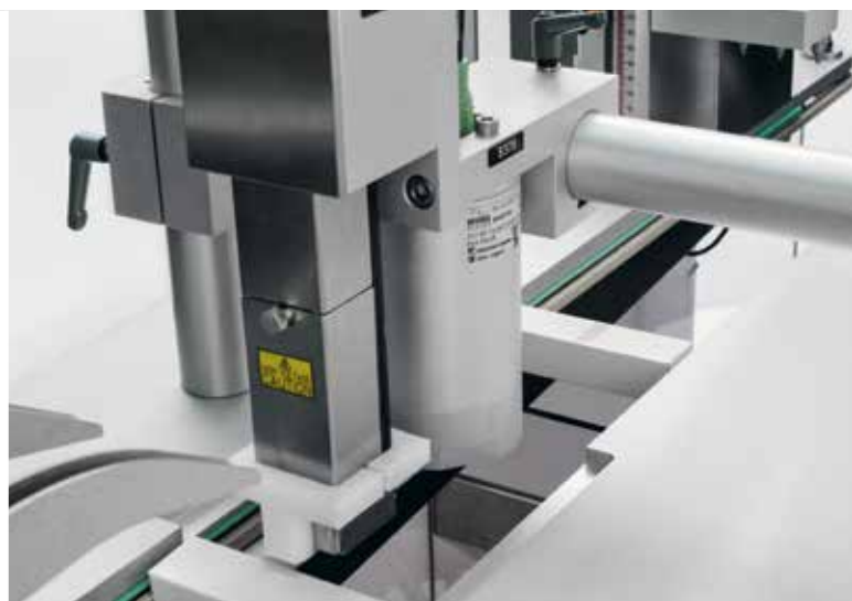
Top printing and camera inspection
