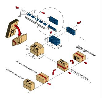
Cartons pre-stacking station collating layers of product during the in-line pusher stokes answers to higher input speed.
