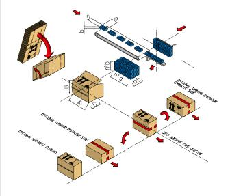
Cartons stacking station in front of the main pusher area – the stacking operation is carried out right in front of the erected case.
