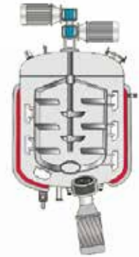
Double way mixing & internal circulation
