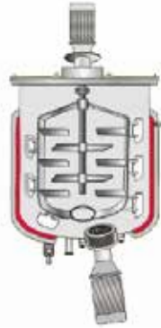
Single way mixing & internal circulation
