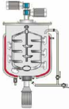
Double way mixing & external circulation
