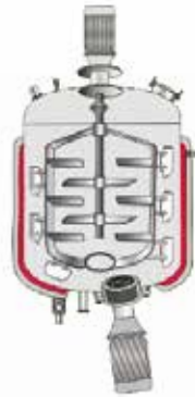
Single way mixing & internal circulation
