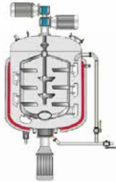
Double way mixing & external circulation
