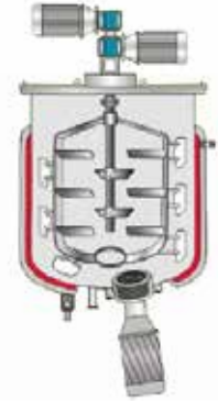
Double way mixing & internal circulation
